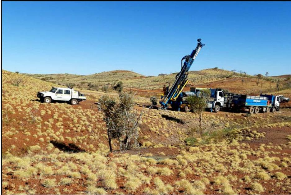
*(Figure 3: RC drilling at Parnell (western sector).)*
