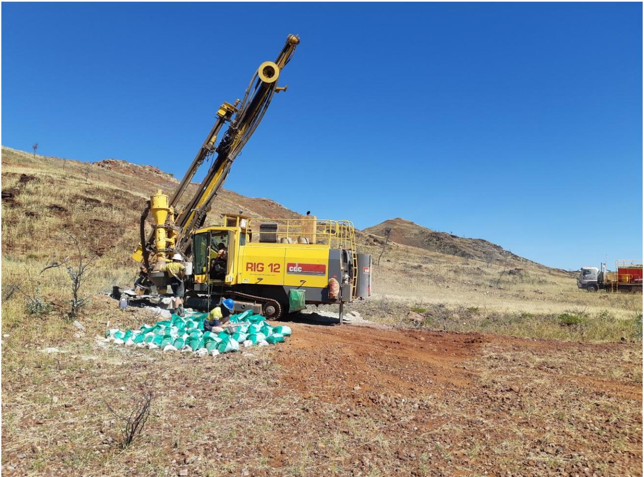
(Figure 4: RC drilling commenced at Talga during July.)
