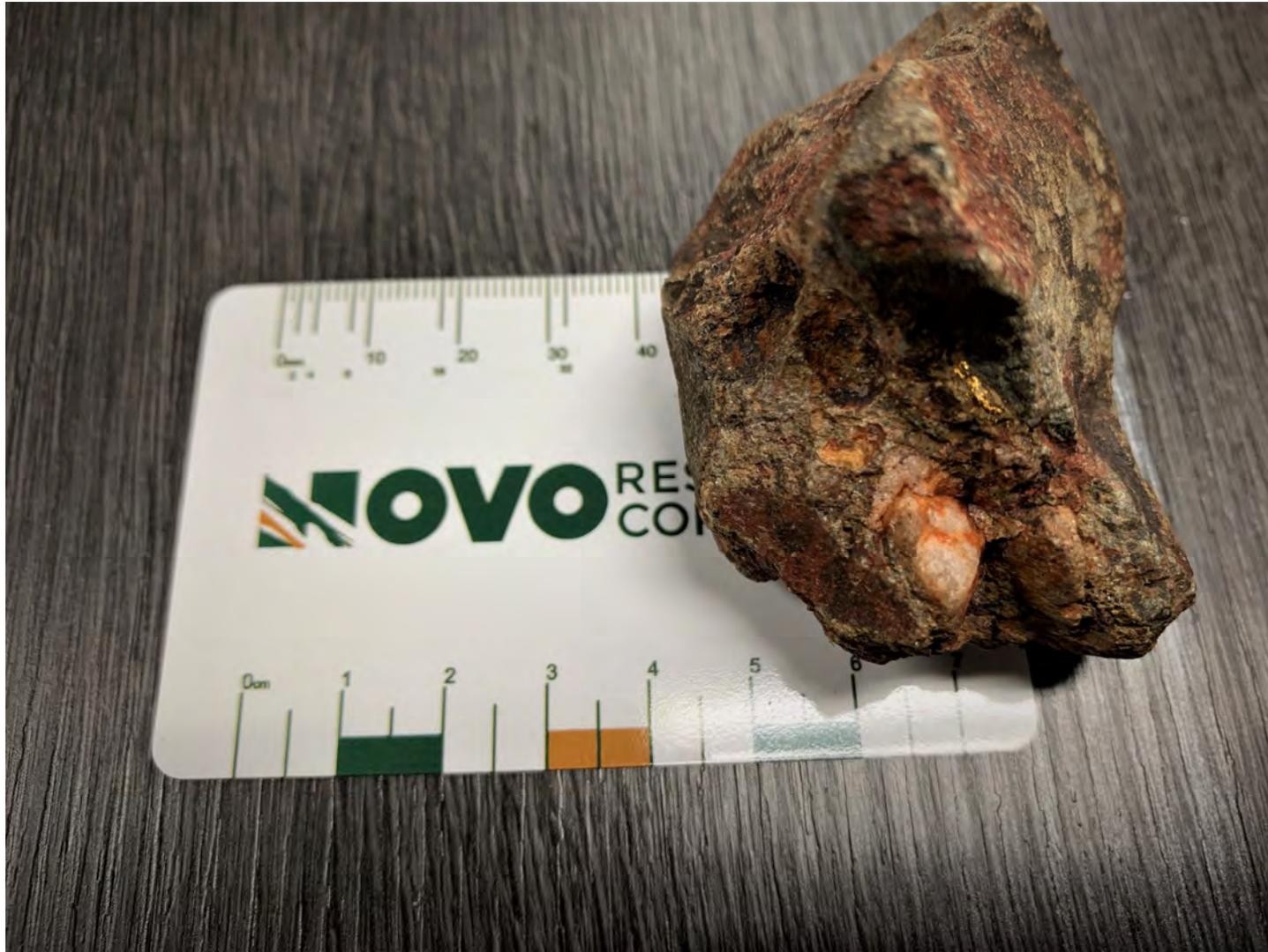
*(Figure 1: Gold recovered from 25-75mm size fraction. The fact that a partial nugget has been detected within a large rock and ejected into concentrate augers well for mechanical sorting as a separation solution. This photograph is of a concentrated gold nugget from approximately 5t of bulk sampled mineralized material and is not necessarily indicative or representative of mineralization hosted on the Comet Well and Purdy's Reward properties.)*
