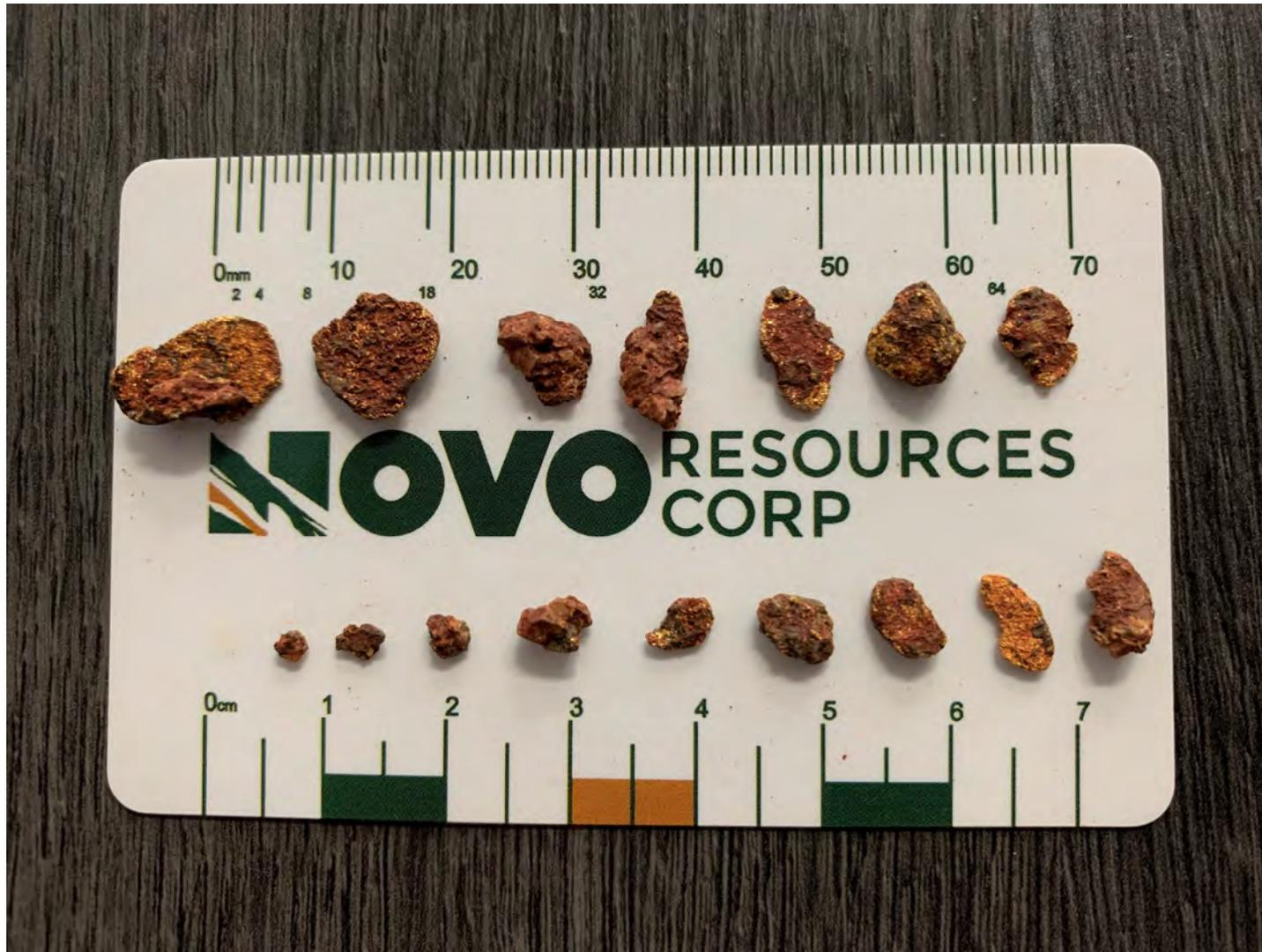
*(Figure 4: Gold recovered from 0-8mm size fraction. Impressively, very fine gold particles encapsulated within rock have been ejected into concentrate from this size fraction. This photograph is of concentrated gold nuggets from approximately 5t of bulk sampled mineralized material and are not necessarily indicative or representative of mineralization hosted on the Comet Well and Purdy's Reward properties.)*
