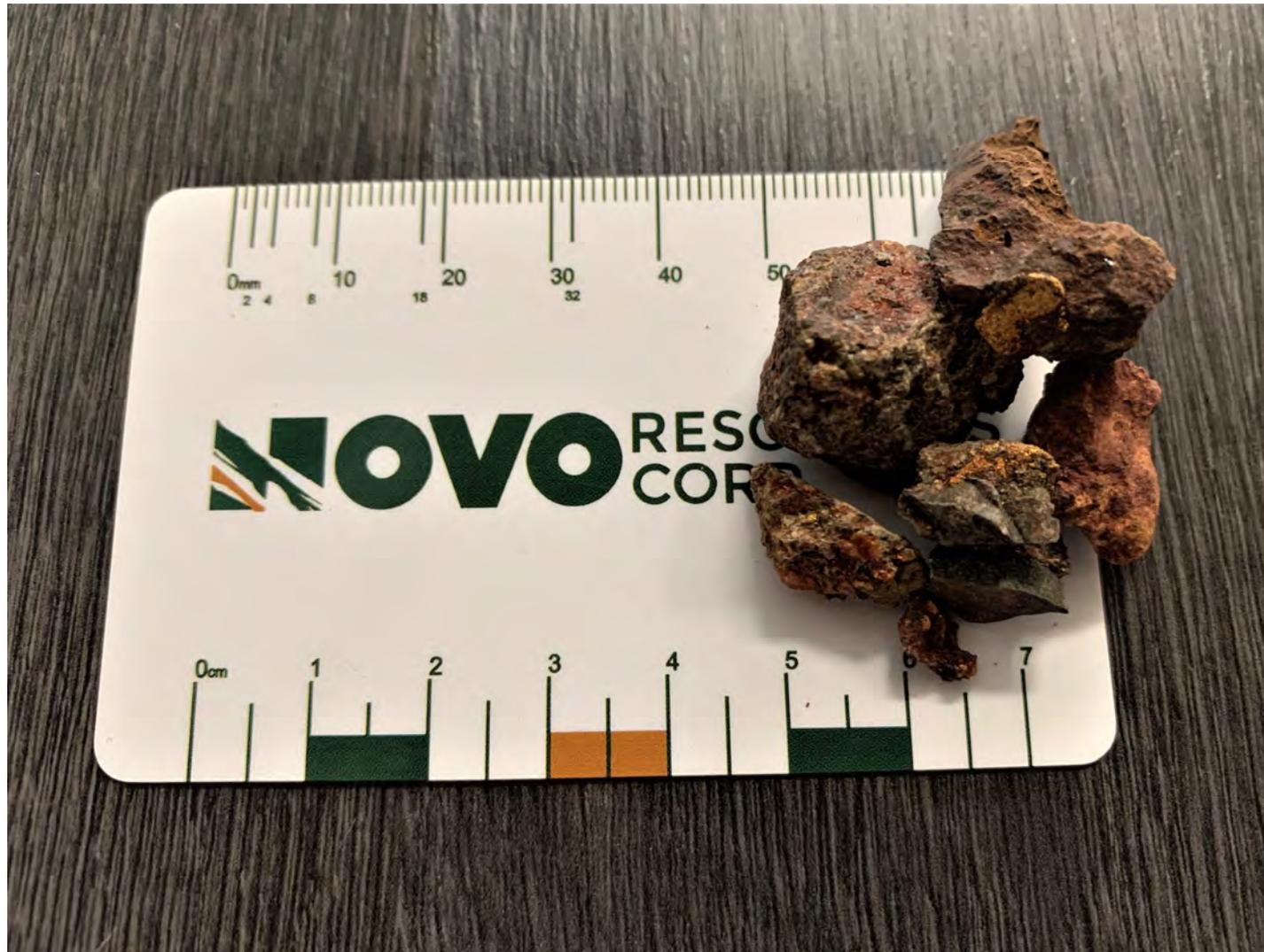
*(Figure 3: Gold recovered from 8-25mm size fraction. Encouragingly, a series of nuggets and separated nugget halos were captured within this size fraction with some very small particles of gold detected within the rocks. This photograph is of concentrated gold nuggets from approximately 5t of bulk sampled mineralized material and are not necessarily indicative or representative of mineralization hosted on the Comet Well and Purdy's Reward properties.)*
