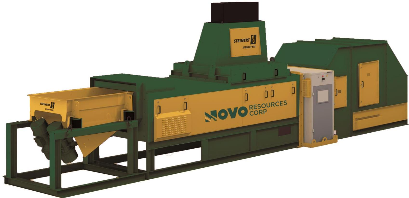
*(Figure 2: Conceptual Steinert mechanical sorter design.)*
