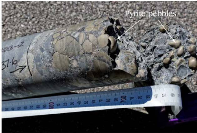
Close-up of coarse pyrite pebbles in conglomerate. Core from hole BCDD13-2 at 37.6 meters. Scale is in millimeters.
