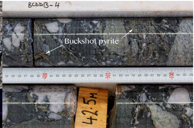
Abundant "buckshot" pyrite grains in conglomerate matrix. Core from hole BCDD13-4 at 42.5 meters. Scale is in millimeters.
